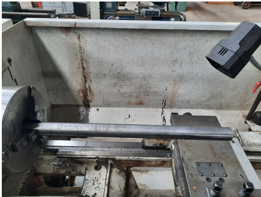
Figure 5.11: Bare Boring Bar Fixed to Lathe
