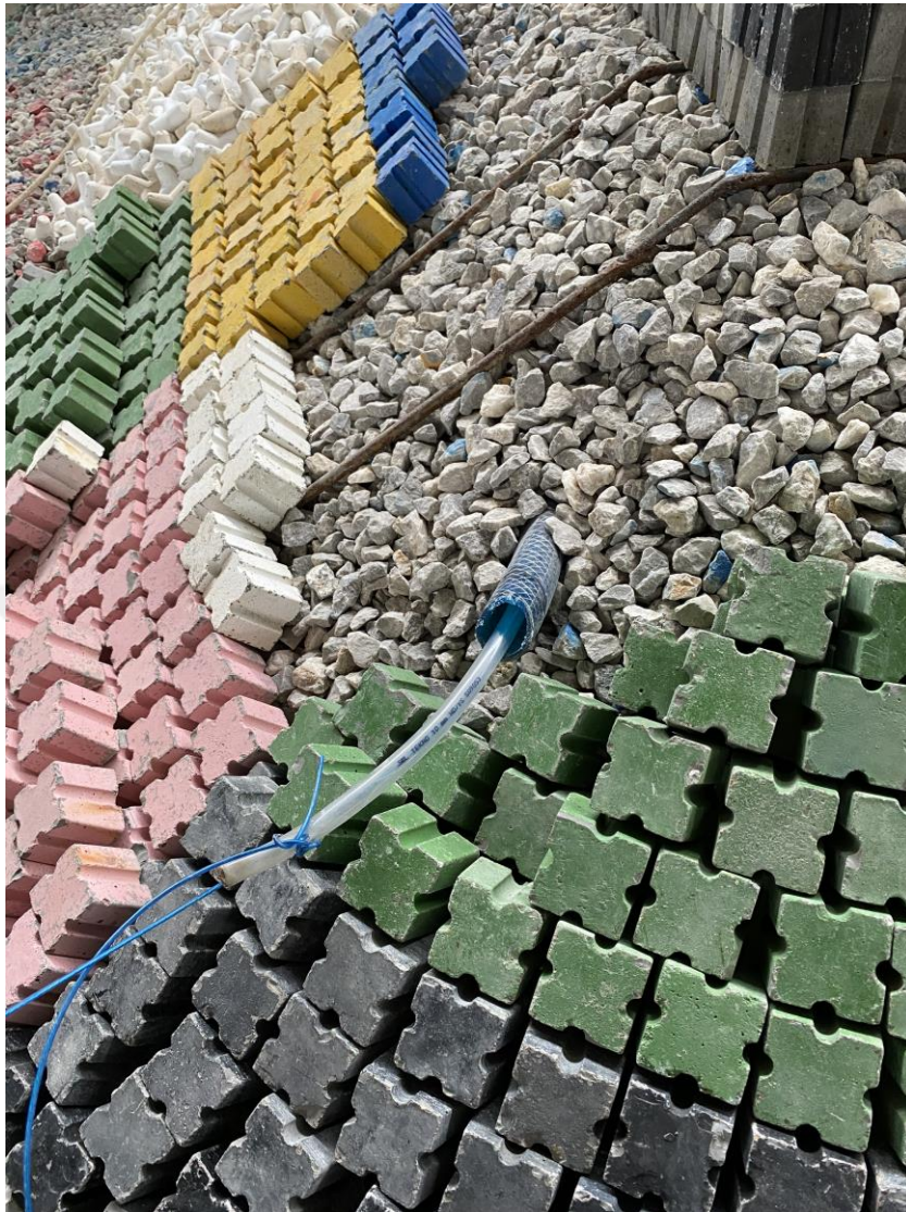
Figure 3.7: Placing process of the hoses inside of the physical model
