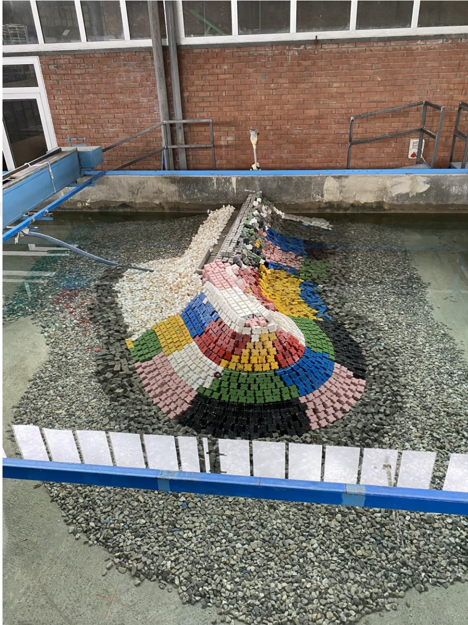
Figure 3.2: Physical model in the wave flume
