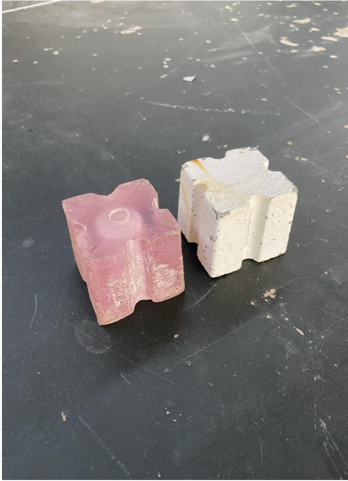
Figure 3.6: Epoxy and concrete antifer units
