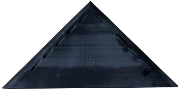
Figure A.4: Nozzle bleed wing narrow CR050 forward ( \Lambda = 45^\circ , t/C = 5.9\% ).
