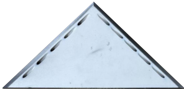
Figure A.3: Nozzle bleed wing wide CR075 ( \Lambda = 45^\circ , t/C = 5.9\% ).
