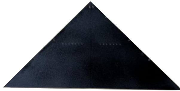
Figure A.6: Blowing wing ( \Lambda = 45^\circ, t/c = 5.9\% )
