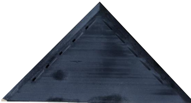
Figure A.5: Nozzle bleed wing narrow CR050 rear ( \Lambda = 45^\circ , t/c = 5.9\% ).
