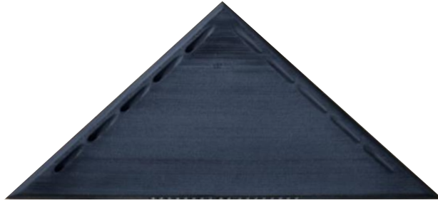
Figure A.2: Nozzle bleed wing wide CR050 ( \Lambda = 45^\circ , t/C = 5.9\% ).
