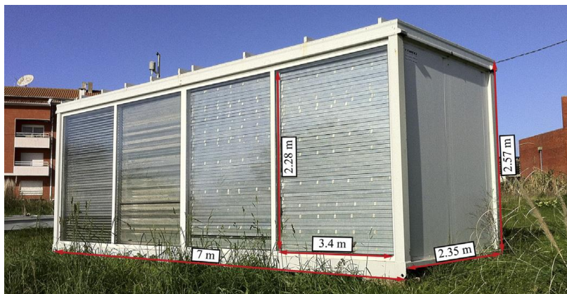
Figure 2.2 PCM Shutter located in Aveiro, Portugal (Silva et al, 2015)
