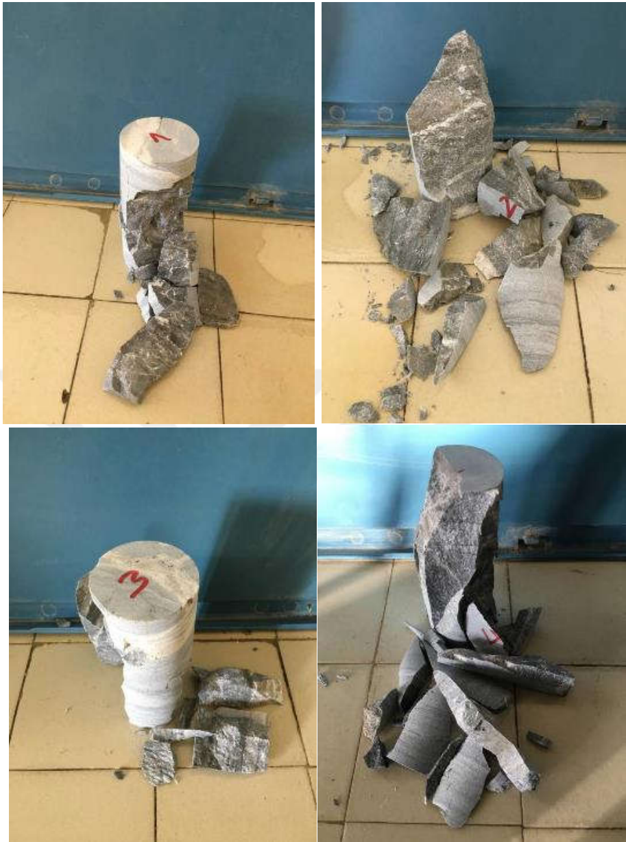
Figure 29. Kuy4 Core Samples UCS and Static Deformability Post-experiment view
