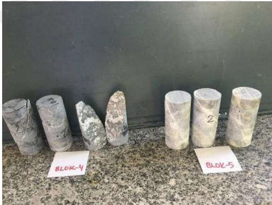
Figure 57. B- 4: İmambaba and B- 5: Halilbeyli core samples – Post-exp.
