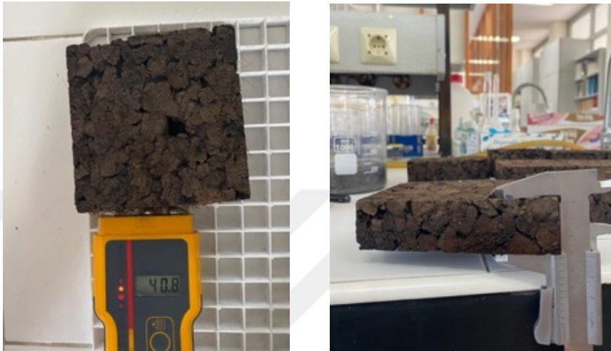
Figure 4.7. Capillary water absorption check with Protimeter and caliper.
