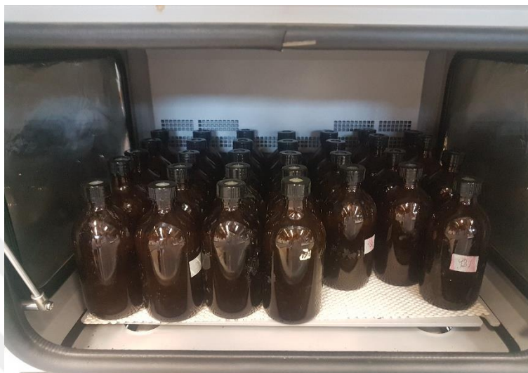
Figure 3.5: The setup of BMP bottles
