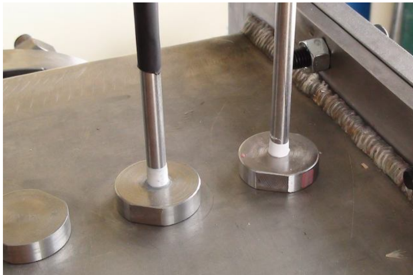
Figure 3-13 Pressure and Temperature Sensor on Combustor
