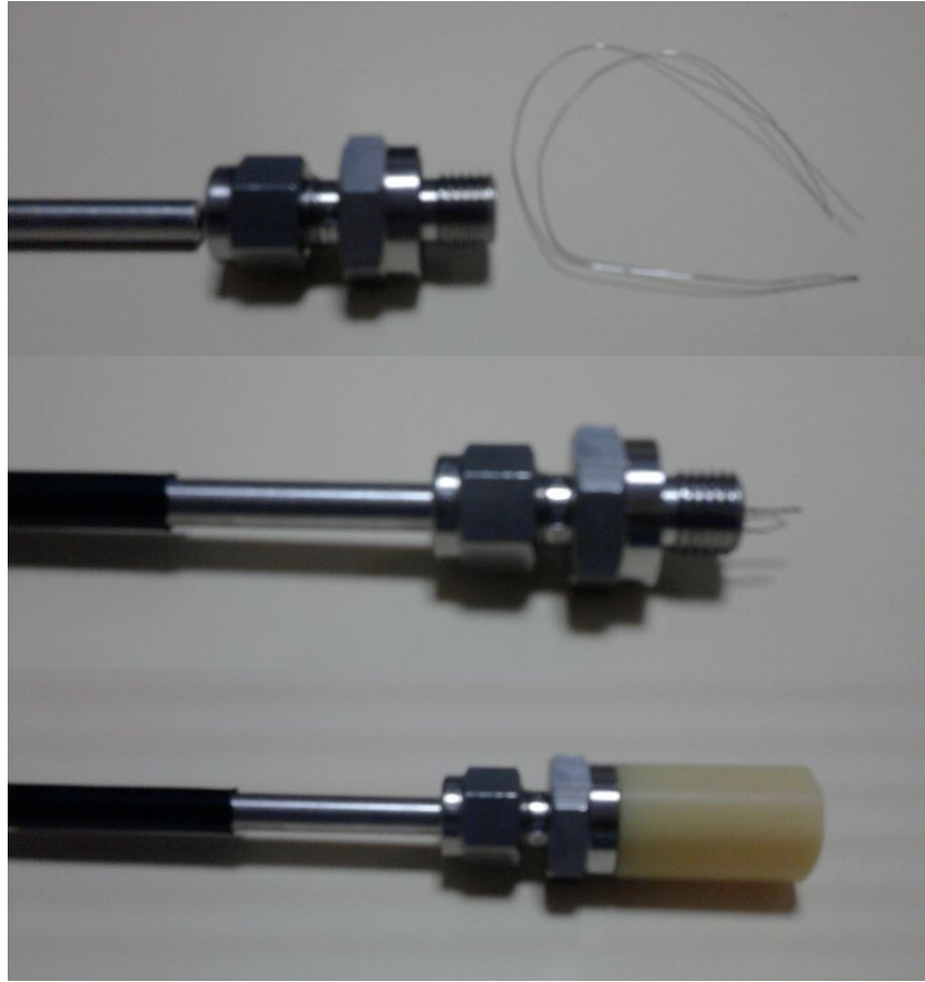
Figure 3-17 Temperature Probe: Parts (top), Assembly (mid), With Cap (bottom)
