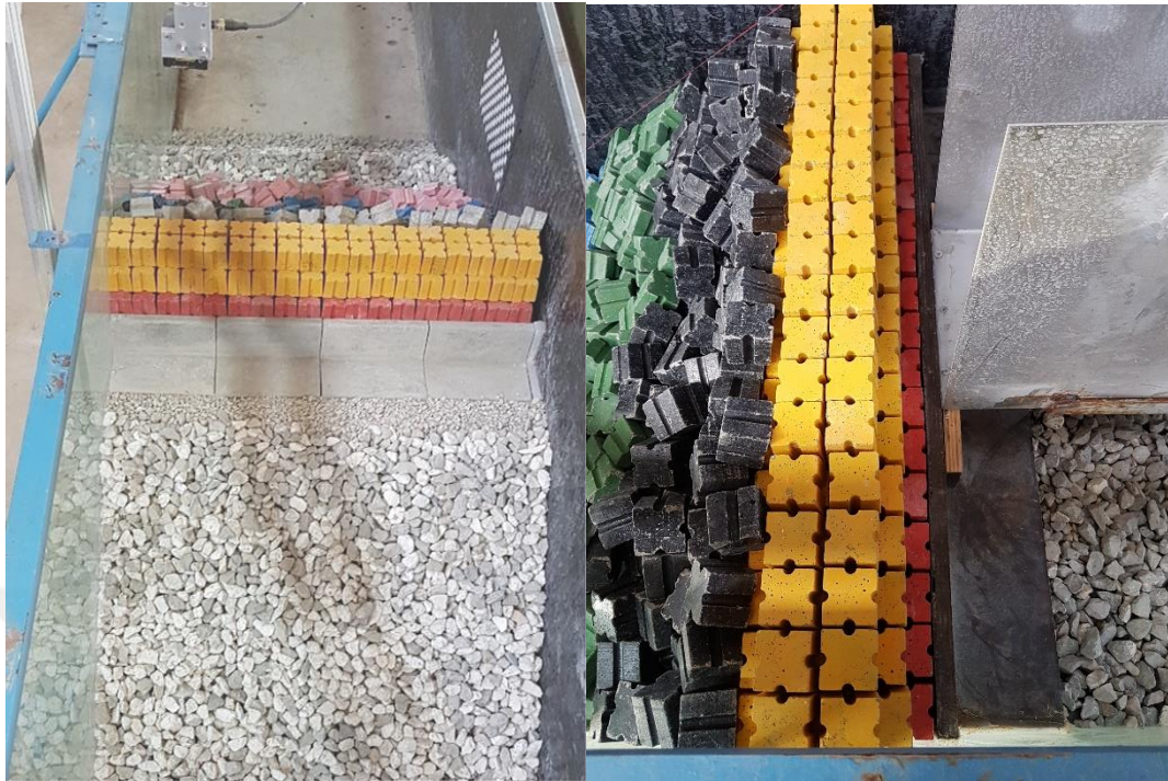
Figure 6.2: Regularly placed antifer units on the crest
