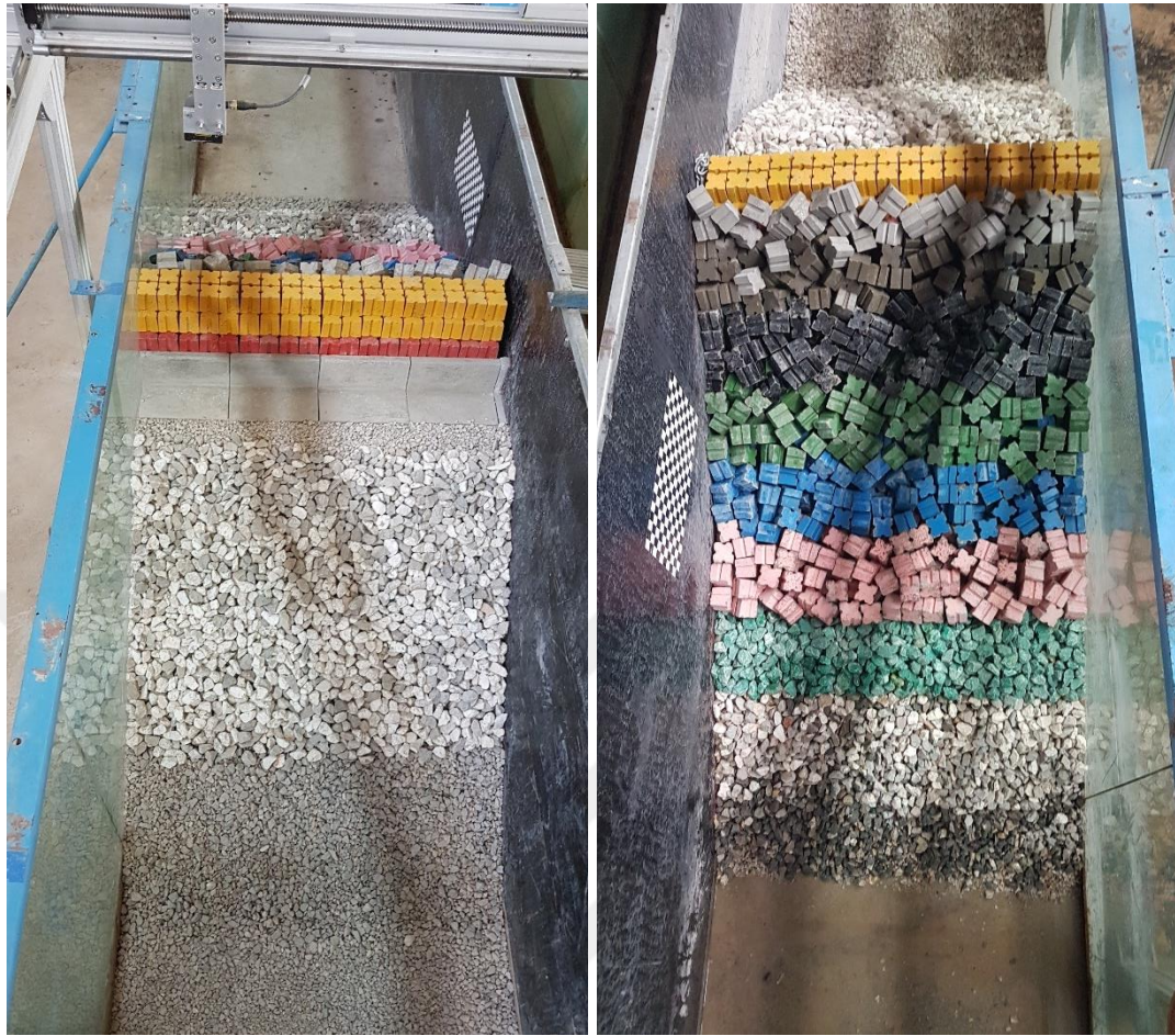
Figure 3.4: Rearside (left) and seaside (right) views of an example cross-section used in the experiments
