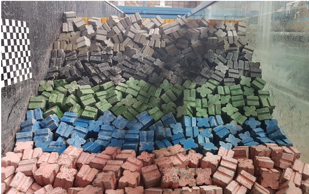
Figure 3.2: Closer look at the seaside view of an example cross-section used in the experiments
