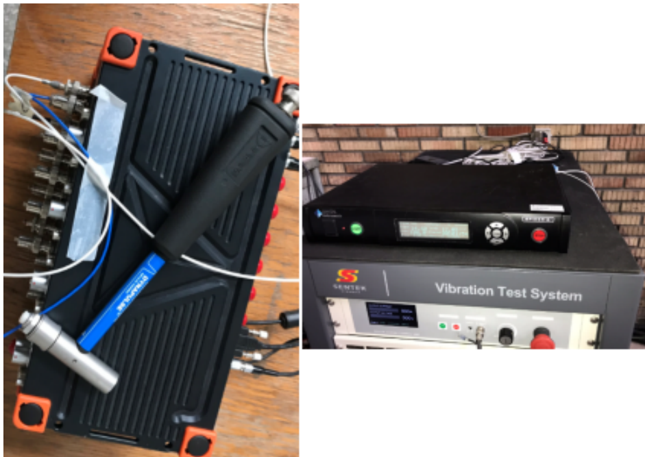
Figure 5.5: Impact Hammer and Vibration Control Device
