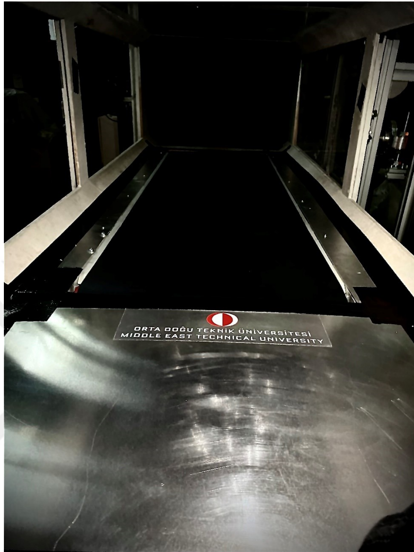
Figure D - 11 Moving belt mechanism inside the wind tunnel test section
