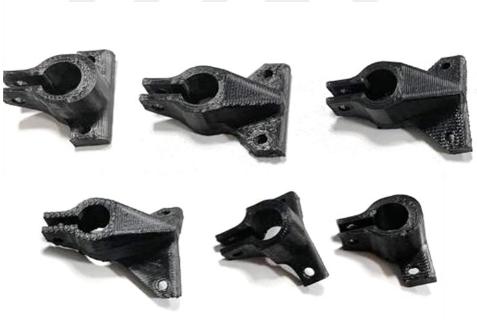
Figure B - 10 Top and perspective views of the 3D printed brackets for thin wings
