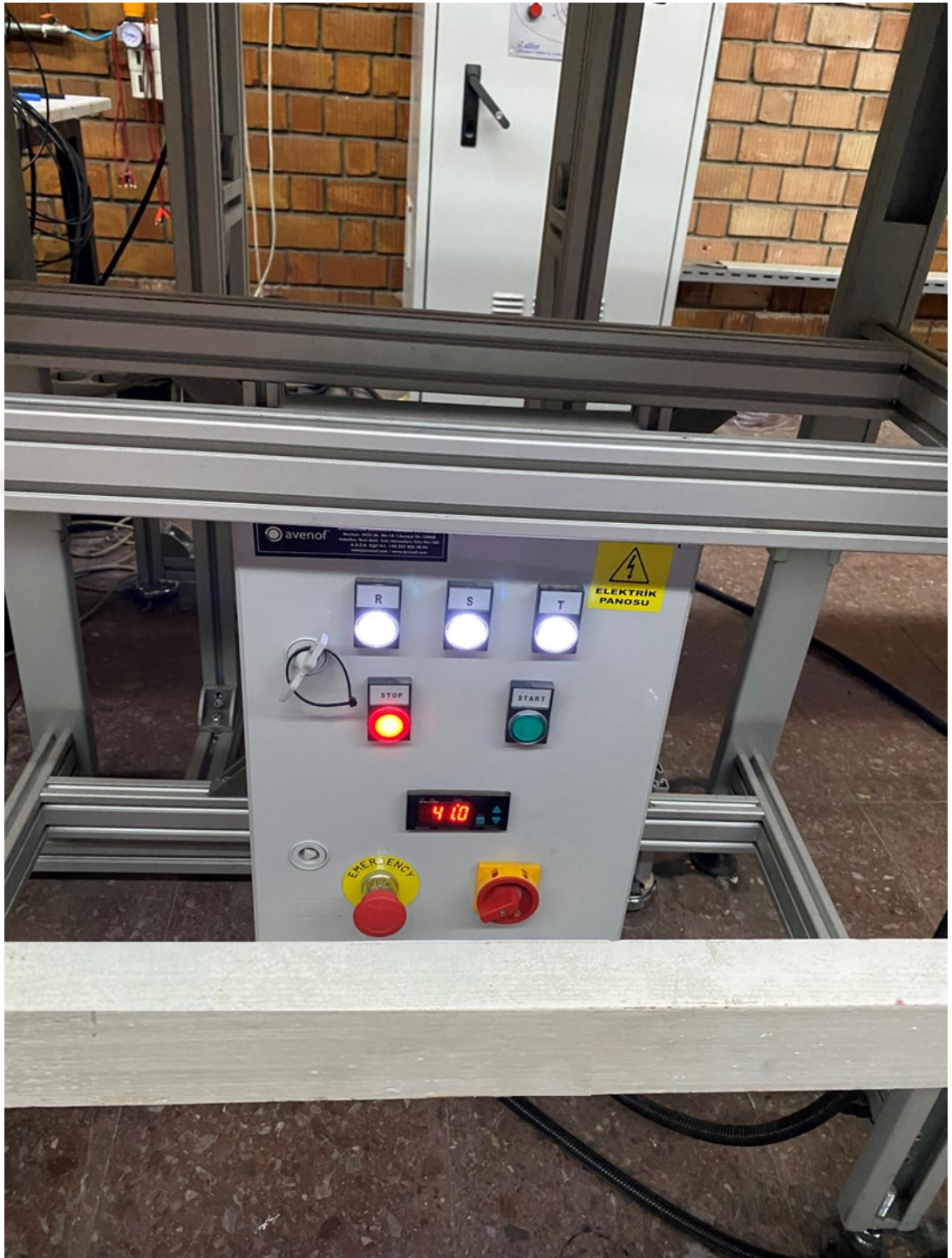
Figure D - 9 Control unit of the moving belt mechanism
