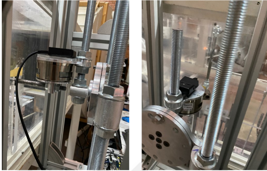
Figure 3-10 The IMU sensor attached to the sensor ground adaptor plate
