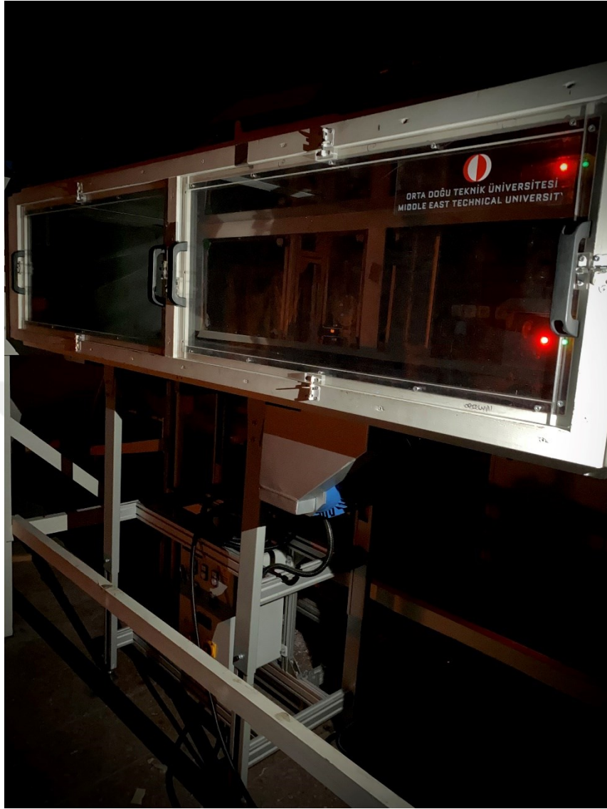
Figure D - 12 Wind tunnel test section with moving belt mechanism
