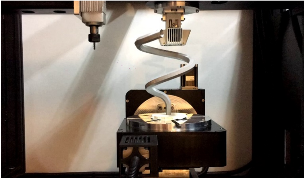
Figure 3.11: Support free printing in 5-axis on Hybro
