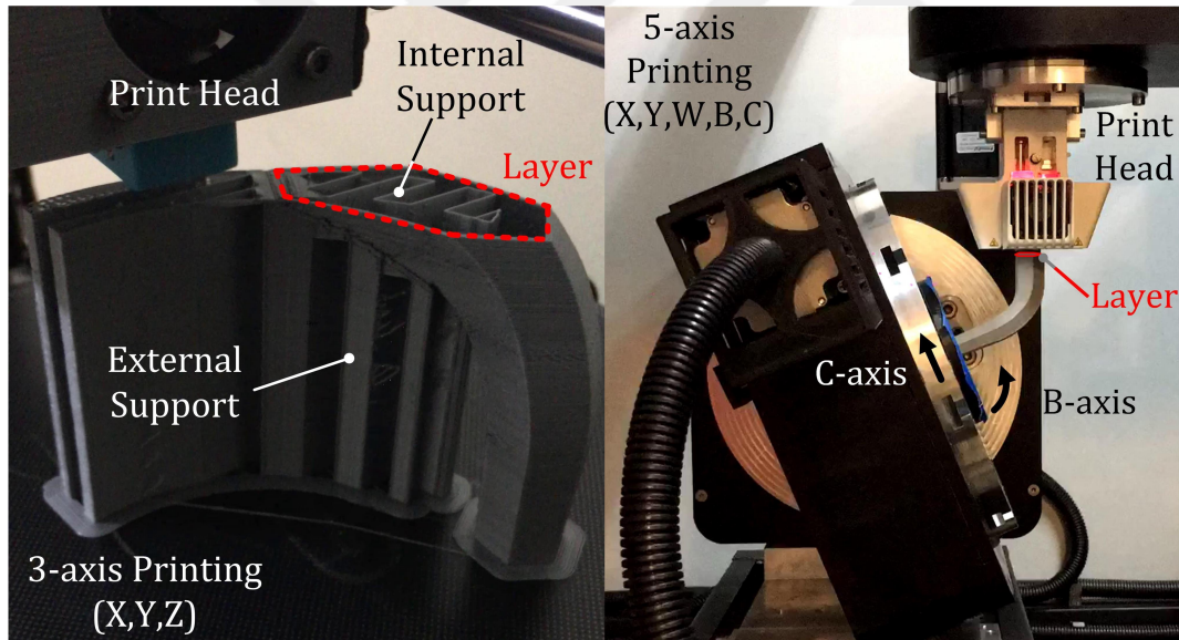
Figure 3.9: Instantaneous captures during manufacturing on 3-axis and 5-axis platforms
