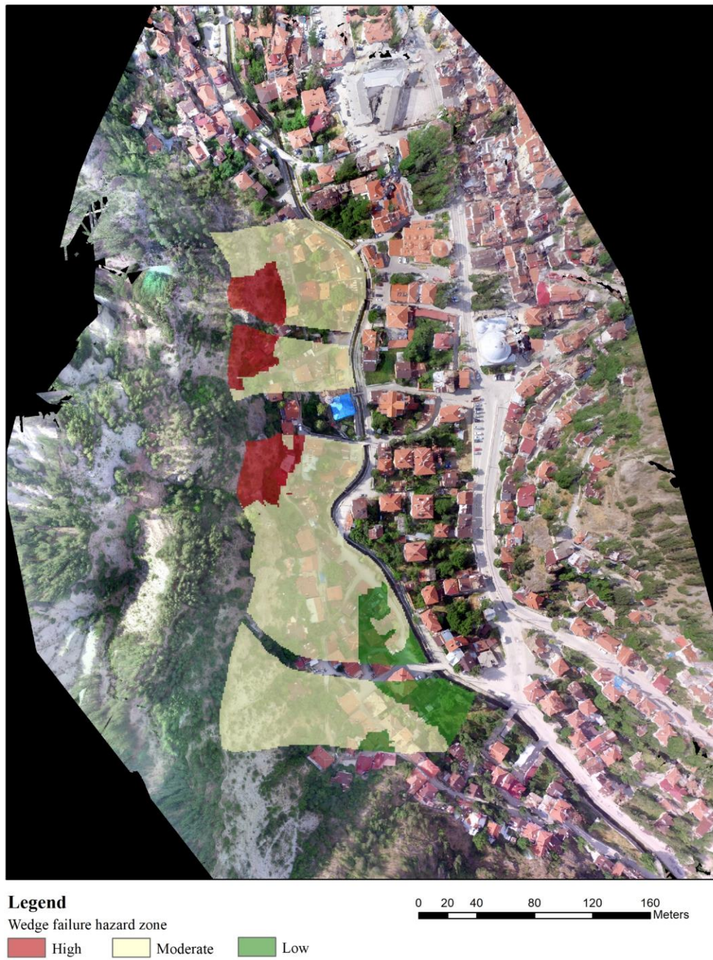
Figure 97: Hazard zonation map of wedge failure on the western side of the Mudurnu valley
