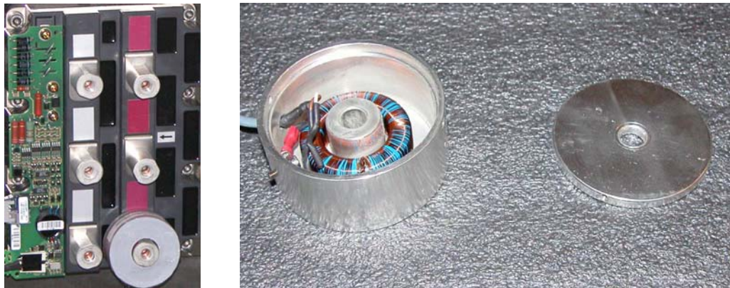
Figure 3.67 CT1 and CT2 Current Transformers
