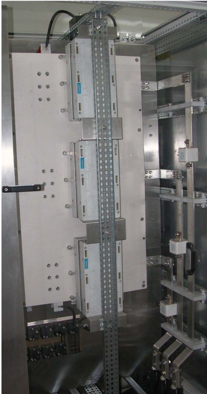
Figure 3.48 DC Link Capacitor Placament in VSC
