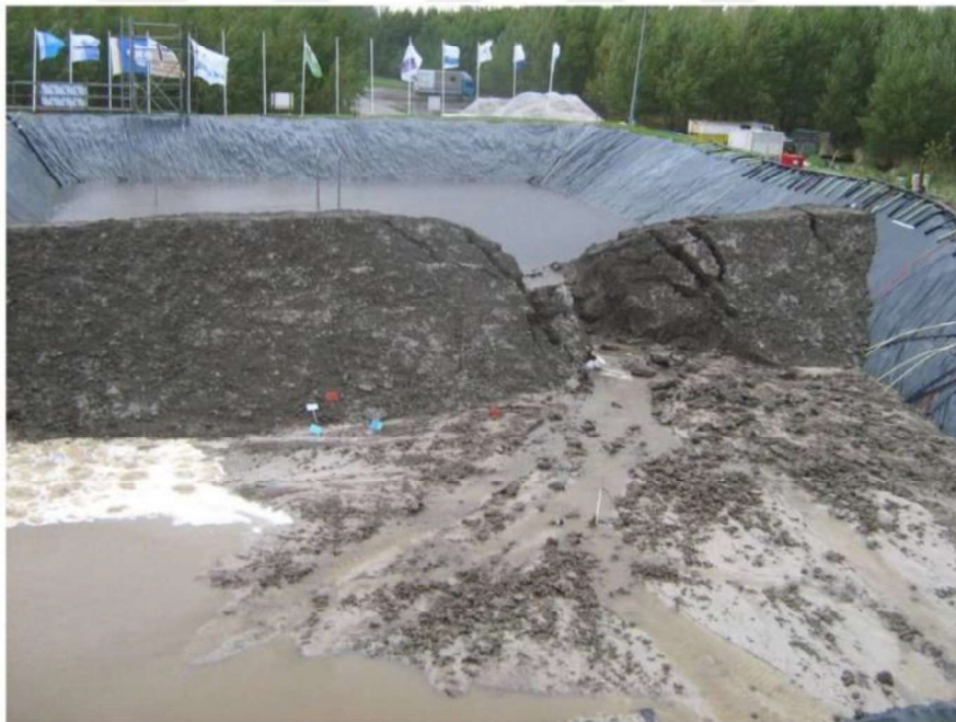
Figure 2.11. Collapse due to backward erosion during Deltares pipe test in the Netherlands (Escaramaia et al. 2013)
