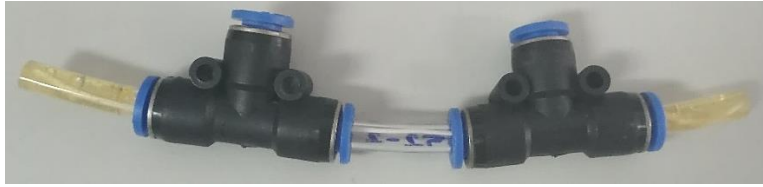
Figure 2. 4. Hollow fiber membrane module used in the filtration tests
