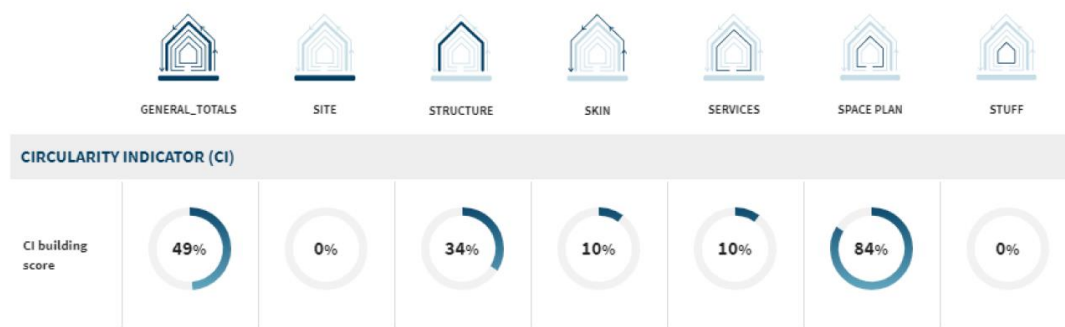
Figure 2.11 Building Layers and Circularity Score in Madaster (Madaster Foundation, 2021)
