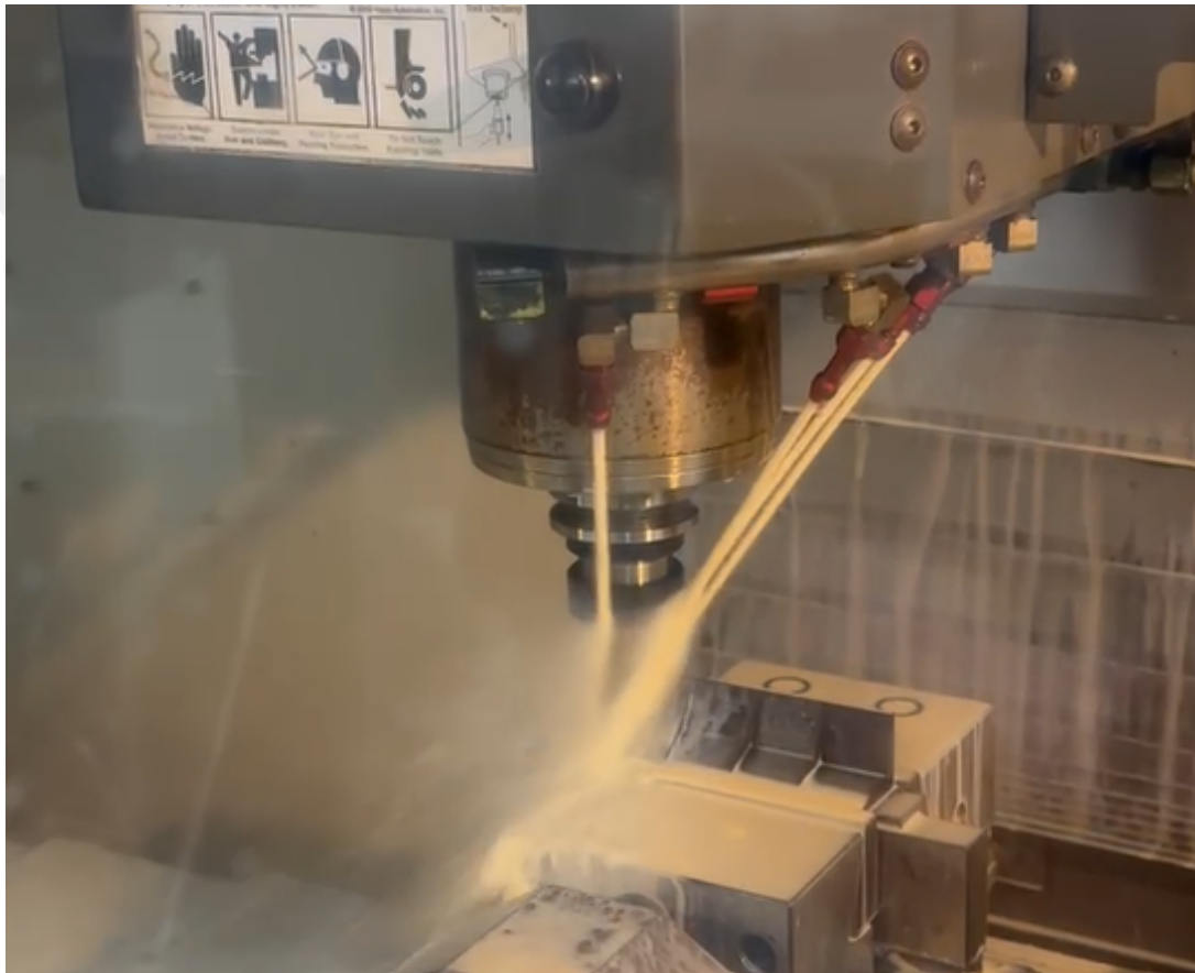
Figure 3.55: Wet Machining Conditions with Fluid Coolant
