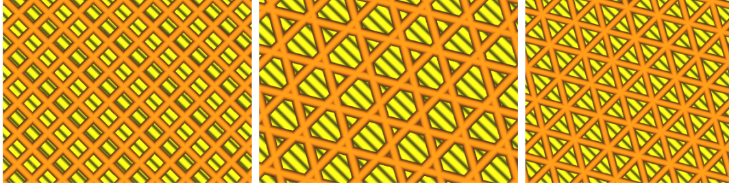
Figure 3.8: Infill Patterns: Left - Grid, Middle - Cubic, Right - Triangle
