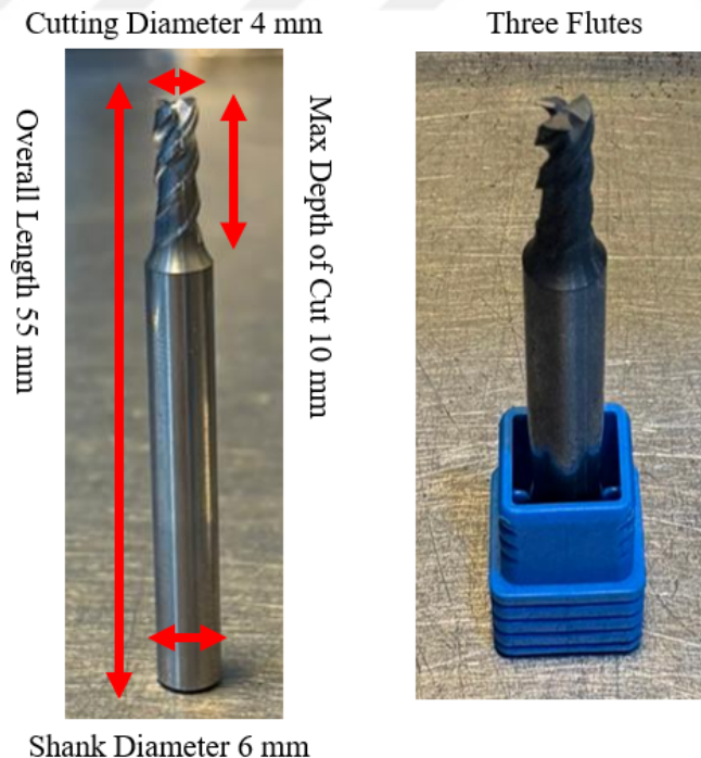
Figure 3.39: 3 Flutes End Mill
