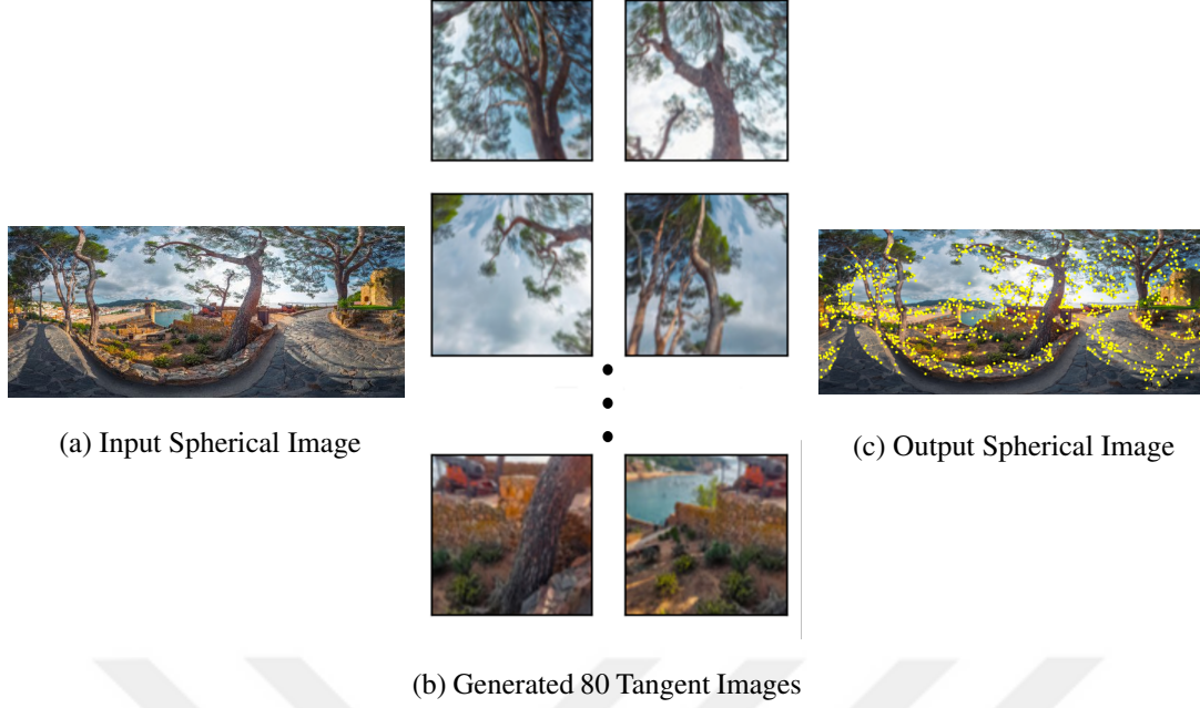
Figure 2.4: Tangent Image Generation & Local Feature Matching Process
