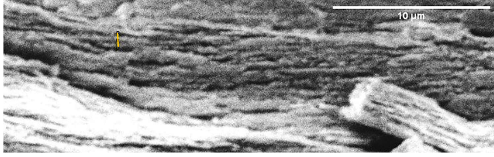
Figure B-1. Cross-section SEM image of the dried sample prepared with the deposition of 0.30% TEMPO-CNC without NaCl. Scale bar is 10 \mu\text{m} . Yellow line represents the cholesteric pitch.
