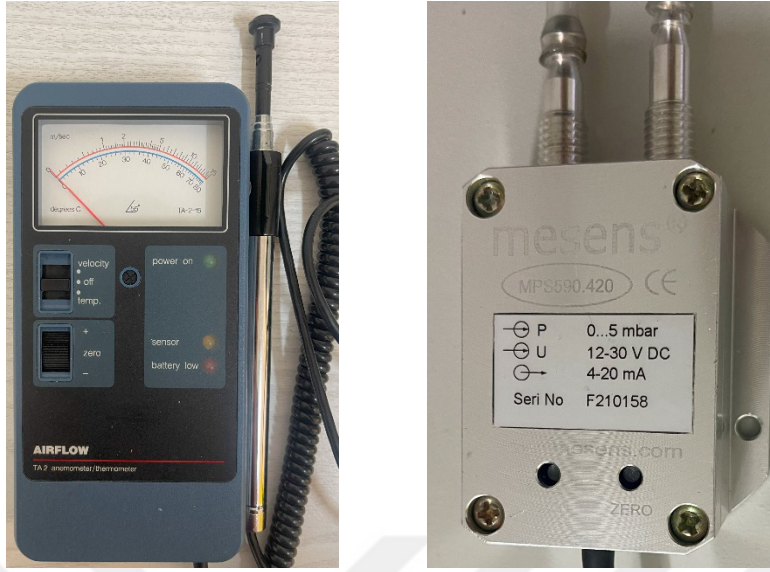
Figure 2.10 Anemometer and differential pressure transmitter
