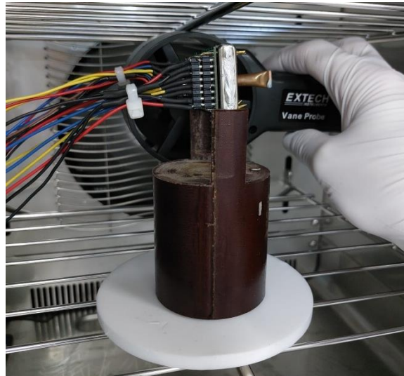
Figure 4.7. Airflow measurement of the climate chamber.
