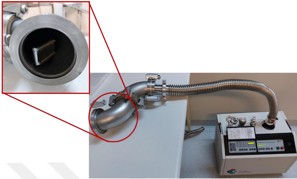
Figure 3.18. Helium leak test setup.
