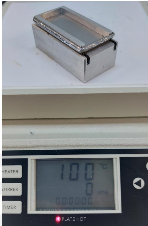
Figure 3.12. The complete soldering operation for edges.
