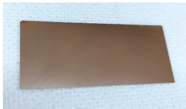
Figure 3.9. Cu deposited side of the alumina substrate
