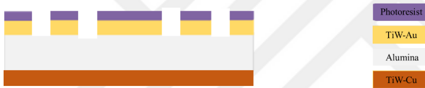
Figure 3.7. TiW/Cu deposited alumina wafer.
