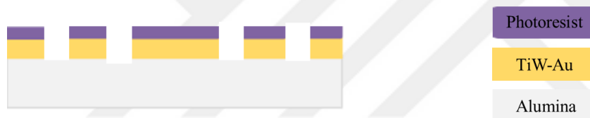
Figure 3.3. TiW/Au is patterned in this step.
