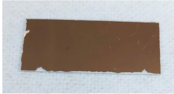
Figure 3.8. Peeled off metal layer.
