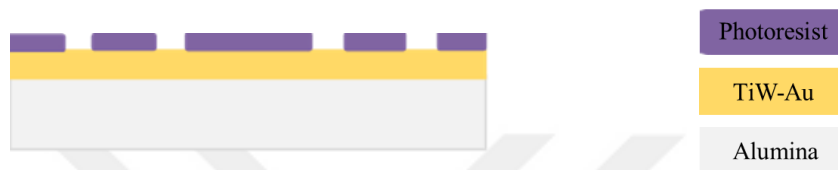
Figure 3.2. Lithography of the alumina wafers.
