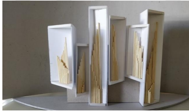
Figure 4.23- 1:50 Scale organ model for acoustic tests, Uygur Architecture archive.
