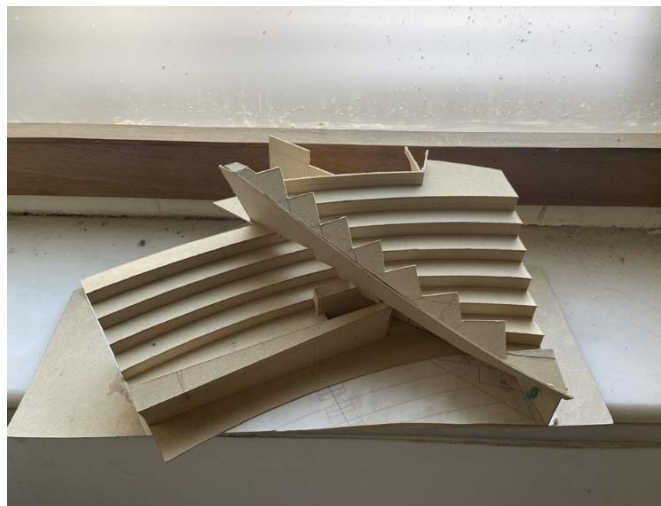
Figure 4.16- 1:50 Scale model where level relationships are studied, photography by the author.
