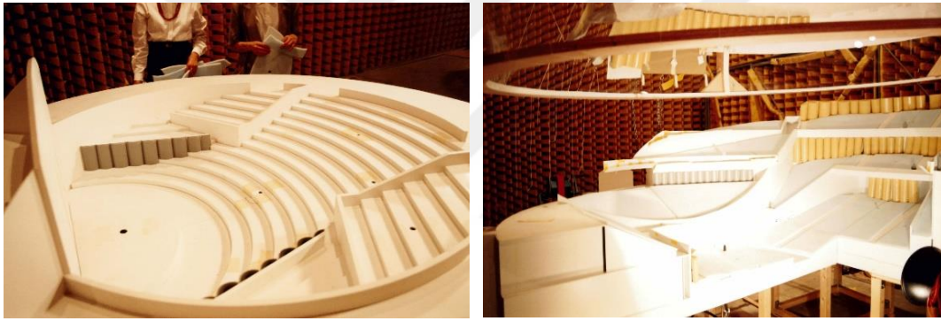
Figure 4.20- Interior of the 1:20 main and chamber music concert hall models built in Germany for acoustic tests, Uygur Architecture archive.
