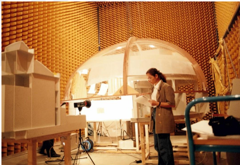
Figure 4.10- Examination of 1:20 Scale model of the main concert hall built for acoustic tests in Germany, Uygur Architecture archive.
