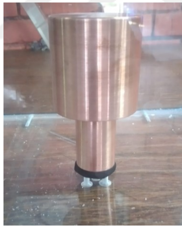
Figure A.4 Copper heater housing placement
