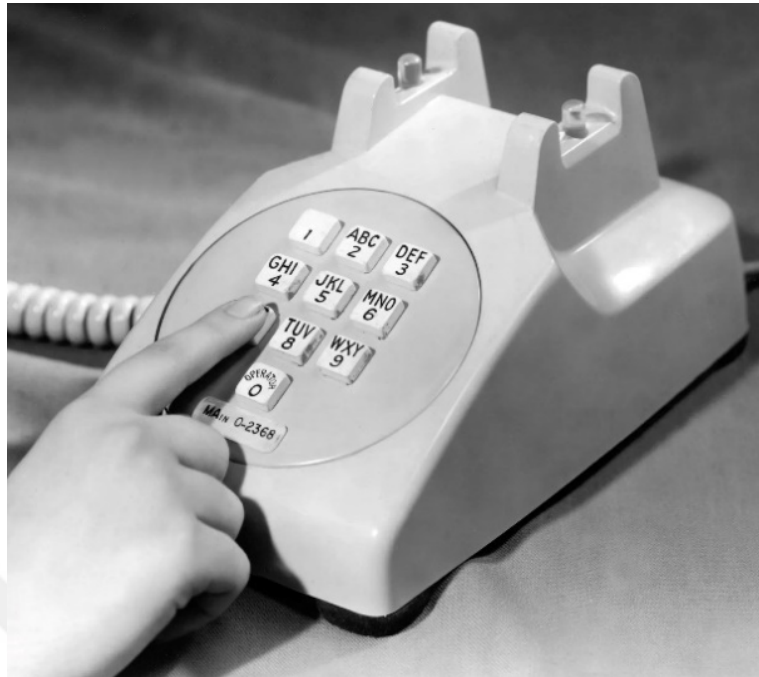
Figure 2.3. 1959 Experimental touch-tone phone model, Bell Labs. (Retrieved from www.nytimes.com/2013/02/09/business/john-e-karlin-who-led-the-way-to-all-digit-dialing-dies-at-94.html?smid=url-share )
