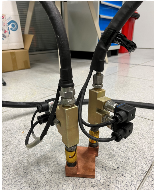
Figure 4.10: Experimental test setup of the cold plates for pressure drop.
