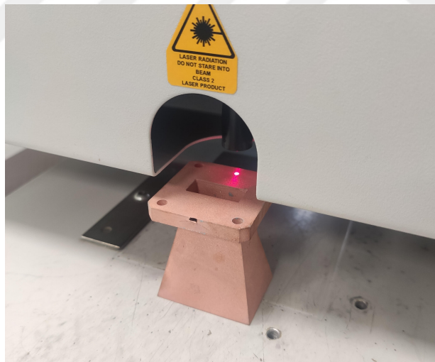
Figure 3.10: X-Ray measurement of the coating thickness
