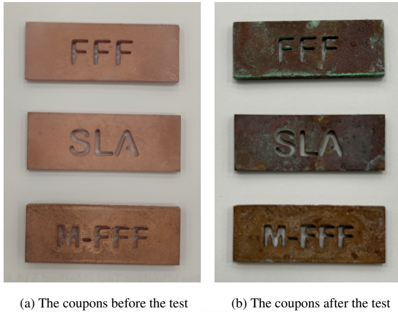
Figure 4.23: Test coupons before and after the salt fog test
