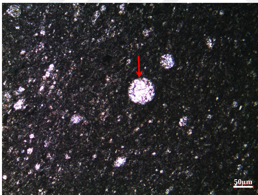
Figure 130. Calcite replaces silica in radiolarian-bearing mudstone microfacies from the thin section at 1697.42 m of the K-11 well
