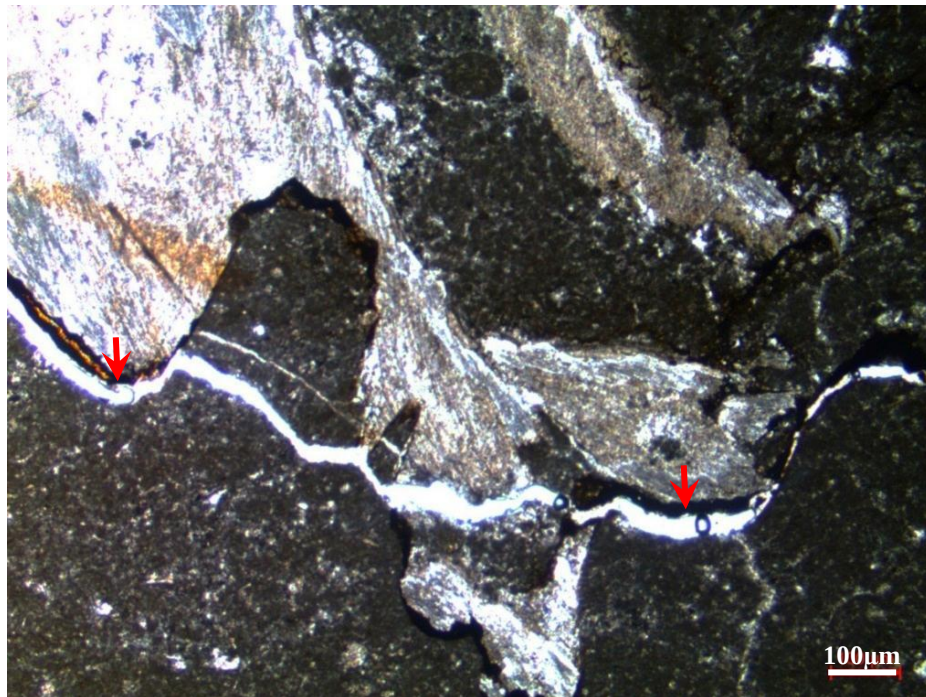
Figure 137. Stylolites formed at around the skeletal fragment from the thin section at 1764.89 m of the K-11 well
