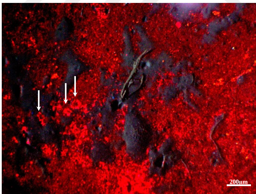
Figure 112. Partially dolomitized recrystallized skeletal fragments and pore spaces, at 1650.69 m of the K-11 well, plane polar light
