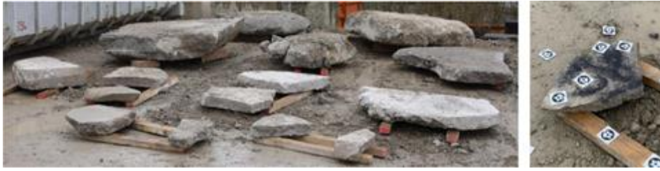
Figure 2.10 The scanning process of the rubble concrete at Tinguely Recycle SA, Vaud, Switzerland (Marshall & Lausanne, 2024)
