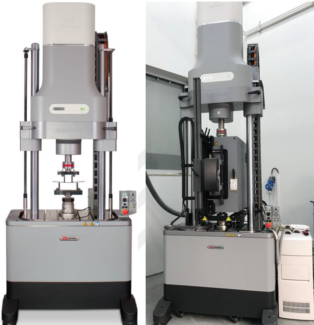
Figure 4.5 Instron® ElectroPuls® E10000 Linear-Torsion All-Electric Fatigue and Dynamic Test Instrument [47].
