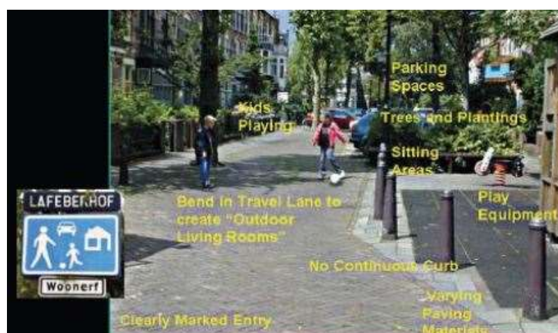
Figure 3.3. Woonerf Design Elements (Appleyard & Cox, 2006, p.31).
