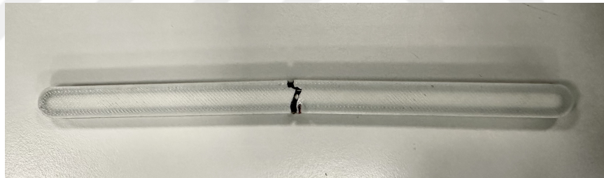
Figure 6.7: Tested bending specimen
