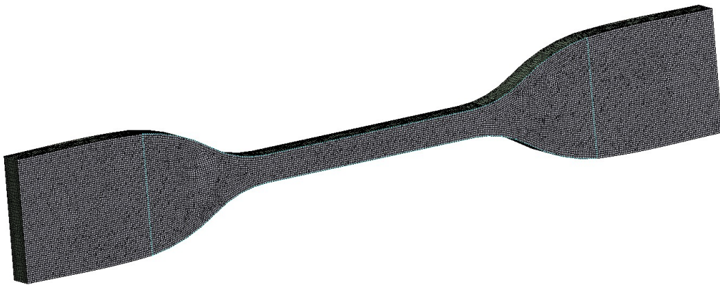
Figure 5.12: 0.5 mm mesh of tensile specimen
