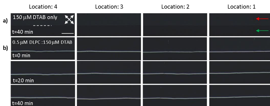
Figure 4.12. Adsorption of DLPC: DTAB mixture into the 5CB-aqueous interface. The polarized optical micrographs are shown that were taken from the 14 \mu\text{m} -deep microfluidic channels where the aqueous phases were composed of (a) 150 \mu\text{M} DTAB, and (b) 0.5 \mu\text{M} DLPC: 150 \mu\text{M} DTAB. Each line of images was collected from locations 1-4 as indicated in the top title. Images were collected at a duration after aqueous phase flow was initiated, as indicated in the images. The white double-sided arrow shows the orientations of the analyzer and polarizers used in all of the images shown in the figure. The dashed lines in the images indicate the location of the horizontal soft interfaces. Scale bar: 100 \mu\text{m} , common for all images.
