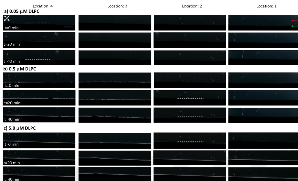
Figure 4.7. Lipid coverage of the interface when lipids are transferred from different concentrations of solutions. Polarized optical micrographs of the microfluidic LC-aqueous interface at locations 1-4 by formed using (a) 0.05 \mu\text{M} , (b) 0.5 \mu\text{M} , and (c) 5.0 \mu\text{M} concentrations of the DLPC feed. Images were collected under a 45^\circ analyzer 135^\circ polarizer. Images were collected at a duration after aqueous phase flow was initiated, as indicated in the images. The white double-sided arrow shows the orientations of the analyzer and polarizers used in all of the images shown in the figure. The dashed lines in the images indicate the location of the horizontal soft interfaces. Scale bar: 100 \mu\text{m} , common for all images. Scale bar: 100 \mu\text{m} .
