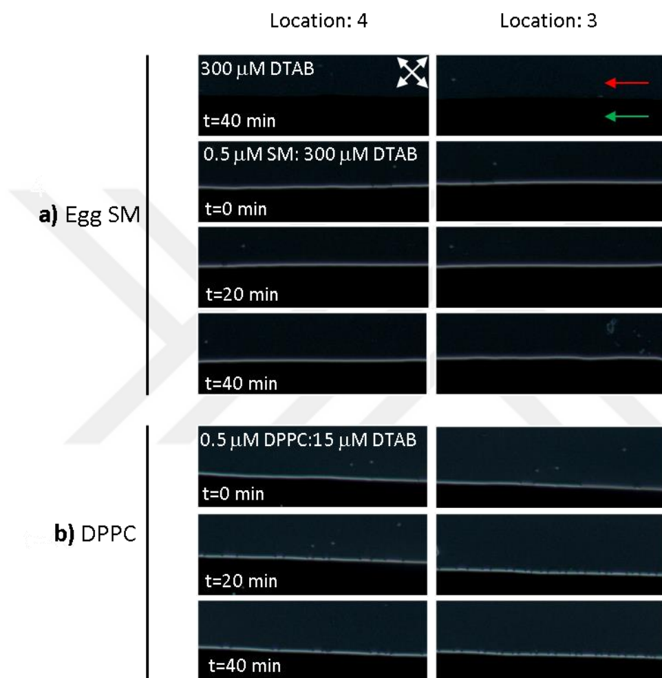
Figure 4.10. Coverage of the interface when lipids are transferred from a mixed solution of surfactants. The polarized optical micrographs are shown that were taken from the 14 \mu\text{m} -deep microfluidic channels where the aqueous phases were composed of vesicles formed by (a) 0.5 \mu\text{M} Egg SM: 300 \mu\text{M} DTAB, and (b) 0.5 \mu\text{M} DPPC: 15 \mu\text{M} DTAB. Each line of images was collected from locations 4 and 3 as indicated in the top title. Images collected from experiments with 300 \mu\text{M} DTAB
