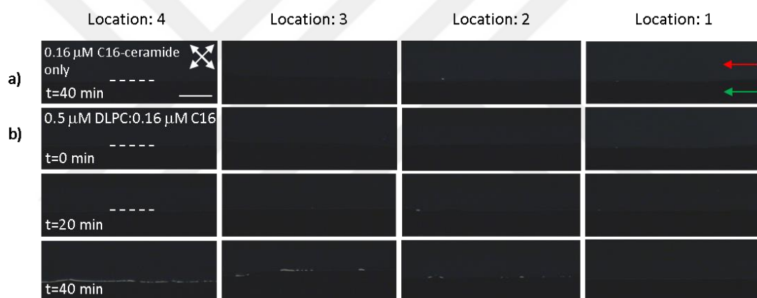
Figure 4.13. Adsorption of DLPC: C16-ceramide mixture into the 5CB-aqueous interface. The polarized optical micrographs are shown that were taken from the 14 \mu\text{m} -deep microfluidic channels where the aqueous phases were composed of (a) 0.16 \mu\text{M} C16-ceramide, and (b) 0.5 \mu\text{M} DLPC:0.16 \mu\text{M} C16-ceramide. Each line of images was collected from locations 1-4 as indicated in the top title. Images were collected at a duration after aqueous phase flow was initiated, as indicated in the images. The white double-sided arrow shows the orientations of the analyzer and polarizers used in all of the images shown in the figure. The dashed lines in the images indicate the location of the horizontal soft interfaces. Scale bar: 100 \mu\text{m} .
