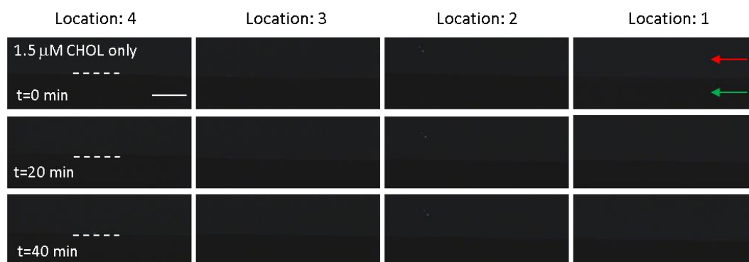
Figure 4.14. 5CB-aqueous phase interface when cholesterol flows as aqueous phase. The polarized optical micrographs are shown that were taken from the 14 \mu\text{m} -deep microfluidic channels, where the aqueous phases were composed of 1.5
