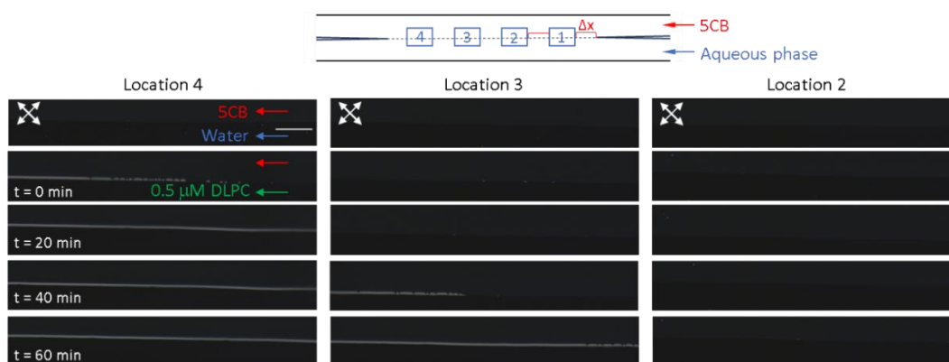
Figure 4.6. Response of the microfluidic, stagnant, and emulsion systems upon adsorption of the DLPC to the interface. The microfluidic channel ( 14\ \mu\text{m} ) is divided into four locations named 1, 2, 3, and 4 for polarized imaging, where \Delta x = 1300\ \mu\text{m} . The polarized optical micrographs of the microfluidic system were taken every ten minutes for one hour, where the aqueous phase was introduced as 0.5\ \mu\text{M} DLPC ( n=8 ).
