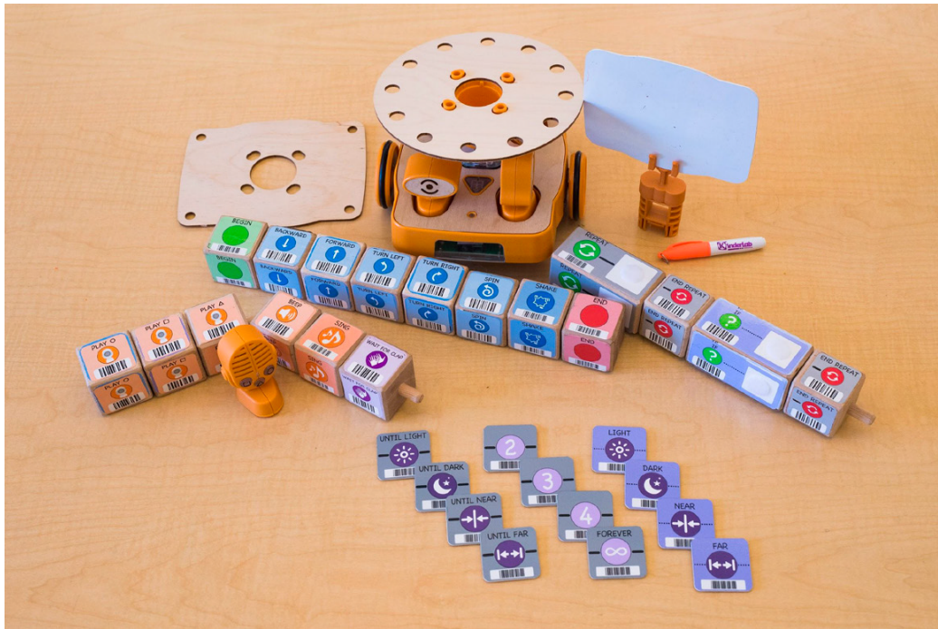
Figure 2. 2. KIBO Robot, Programming Blocks, Sensors, and Parameters
