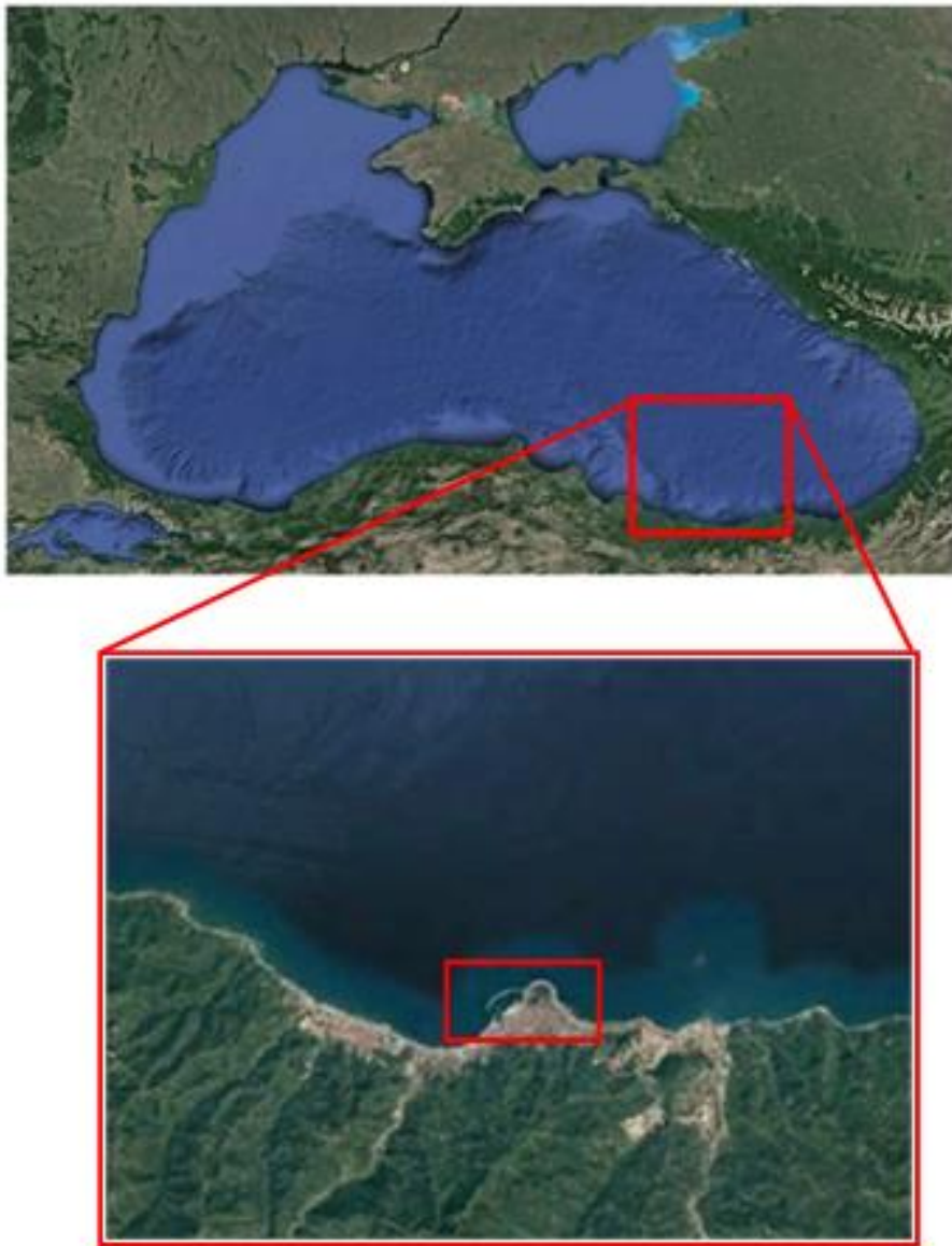
Figure 4.1: Study area, red box in the upper picture covers the ADCIRC+SWAN domain boundaries and red bow in the lower picture covers the NAMI-DANCE domain boundaries
