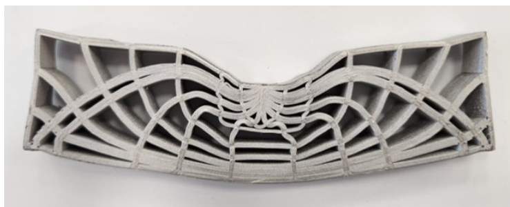
(d) Deformed shape of MBB Beam having optimized infill whose G-code is created by the algorithm
