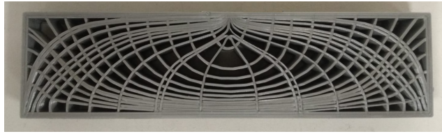
(a) Manufactured part with a layer thickness of 0.6mm
