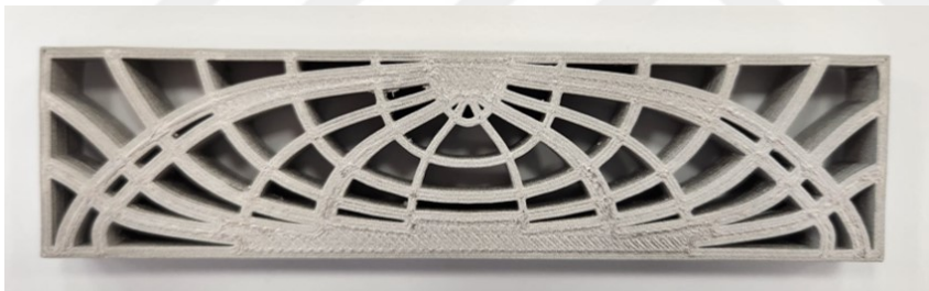
(c) Part 3: MBB Beam having optimized infill whose G-code is created by Cura
