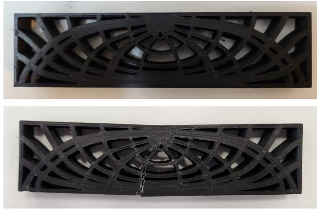
Figure 3.35: MBB Beam Part 8 and its fracture shape
