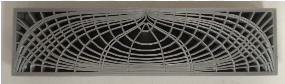
Figure 3.9: The manufactured part with a layer thickness of 0.6 mm
