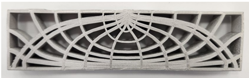
(d) Part 4: MBB Beam having optimized infill whose G-code is created by the algorithm
