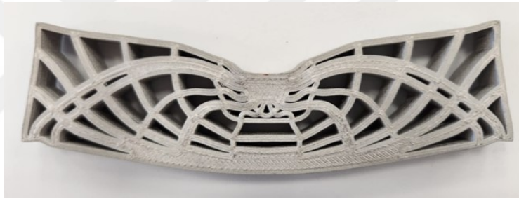
(c) Deformed shape of MBB Beam having optimized infill whose G-code is created by Cura
