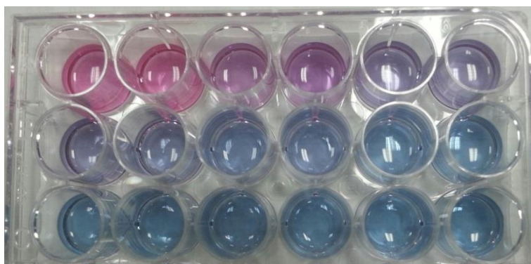
Figure 3.1 Color shift among wells after AB assay following quercetin treatment ranging from 25 \mu M to 200 \mu M.
