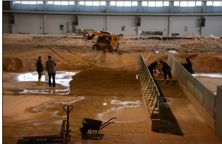
Figure 5.3 Preparing the bottom topography for Rize – Artvin Airport physical modeling
