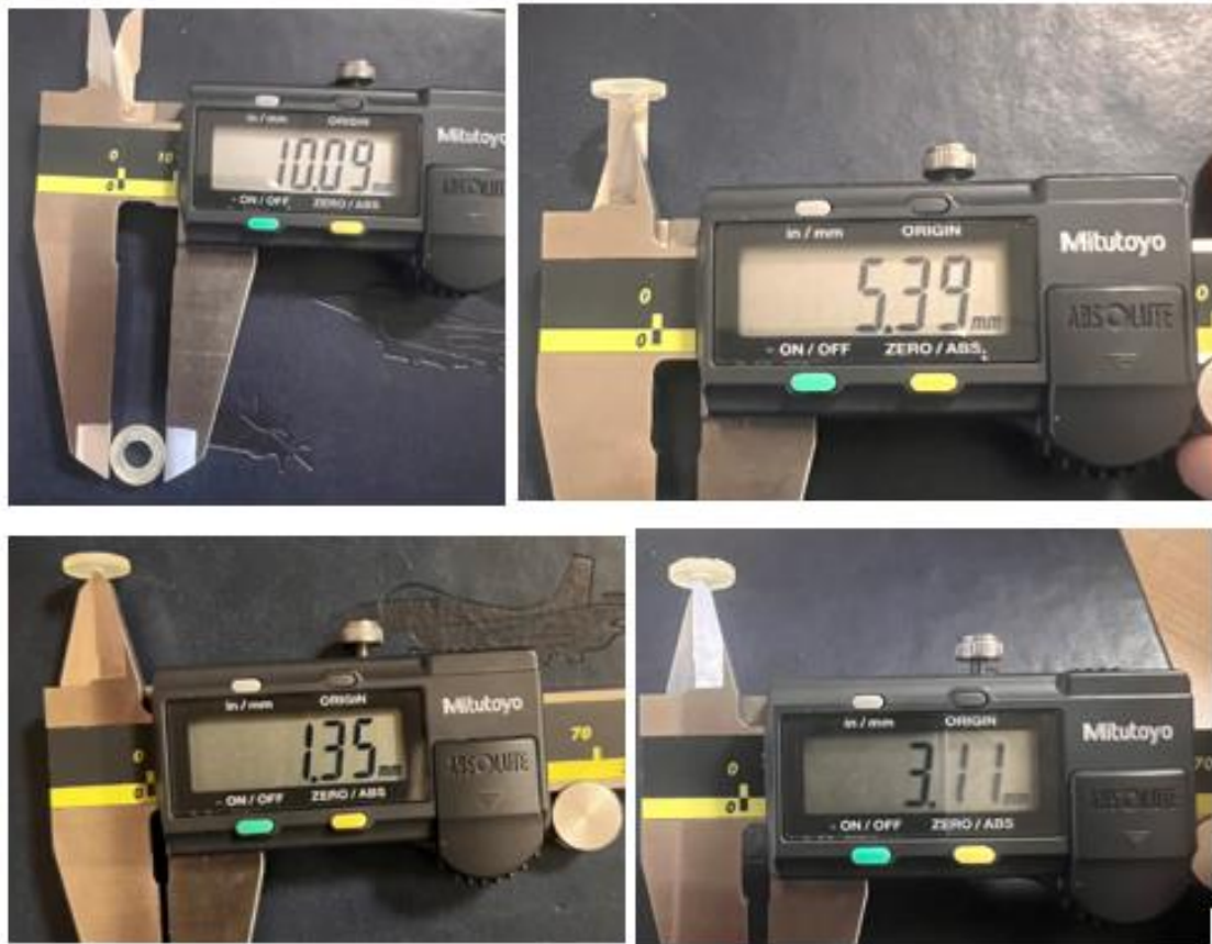
Figure 3.4 99%, 90%, and 70% occlusion sample diameter
