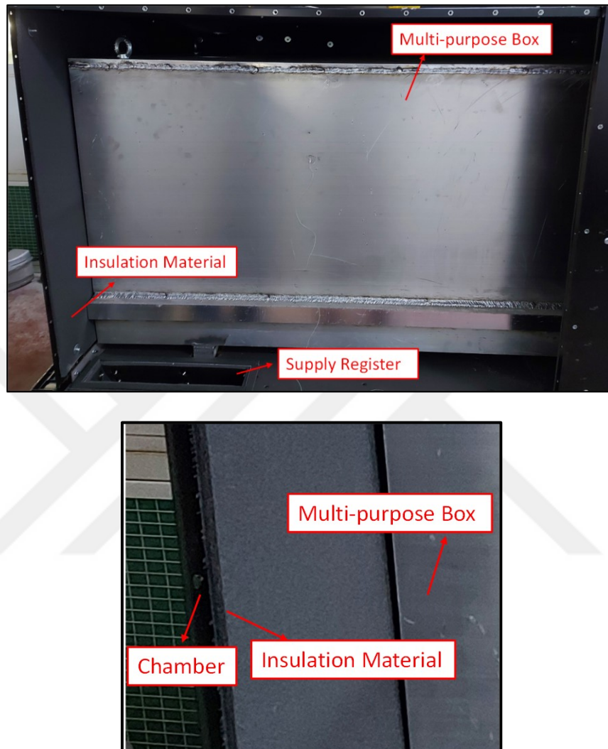
Figure 3-6. Multi-purpose box, supply register and insulation material
