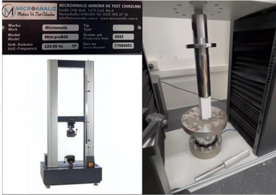
Figure 34. Compression test setup and its specifications (photographs taken by author).
