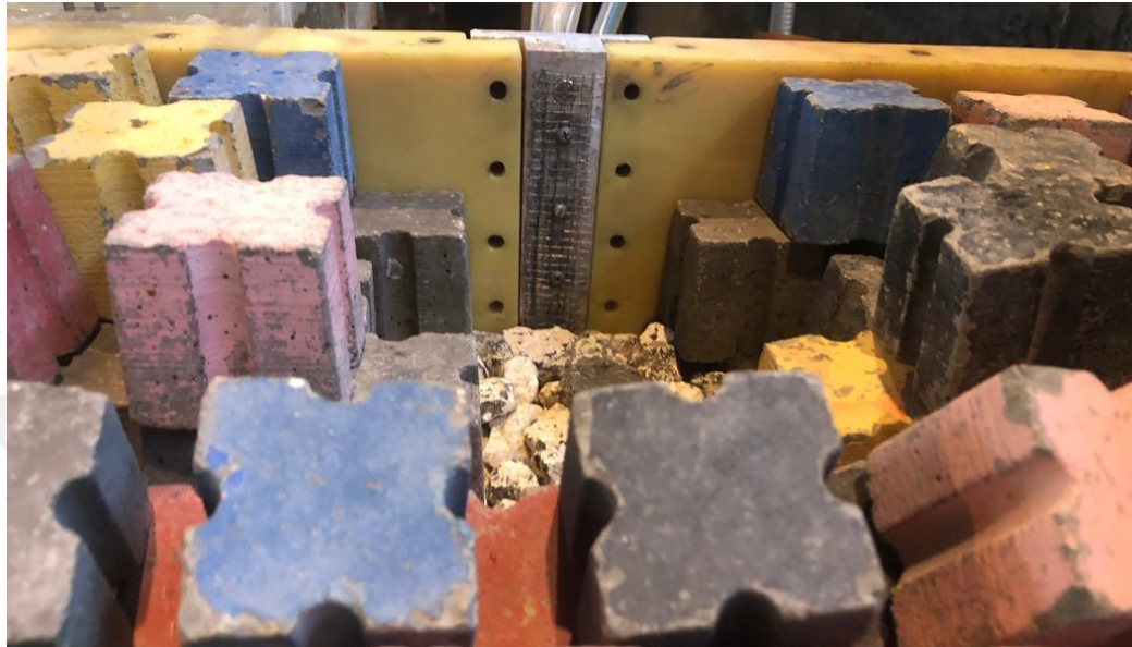
Figure 3.7. Aluminium apparatus position on the vertical face of the crown wall.
