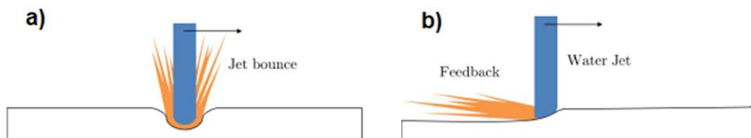
Figure 4.47. Water splashing direction [121]
