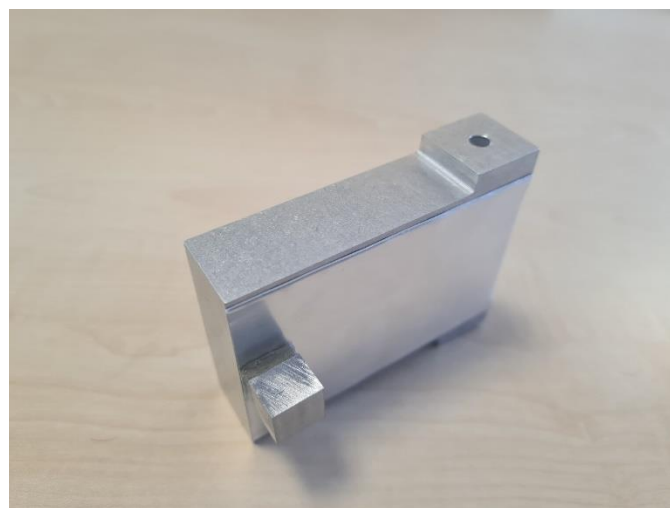
Figure 4.14 General View of One Isolator With TVA
