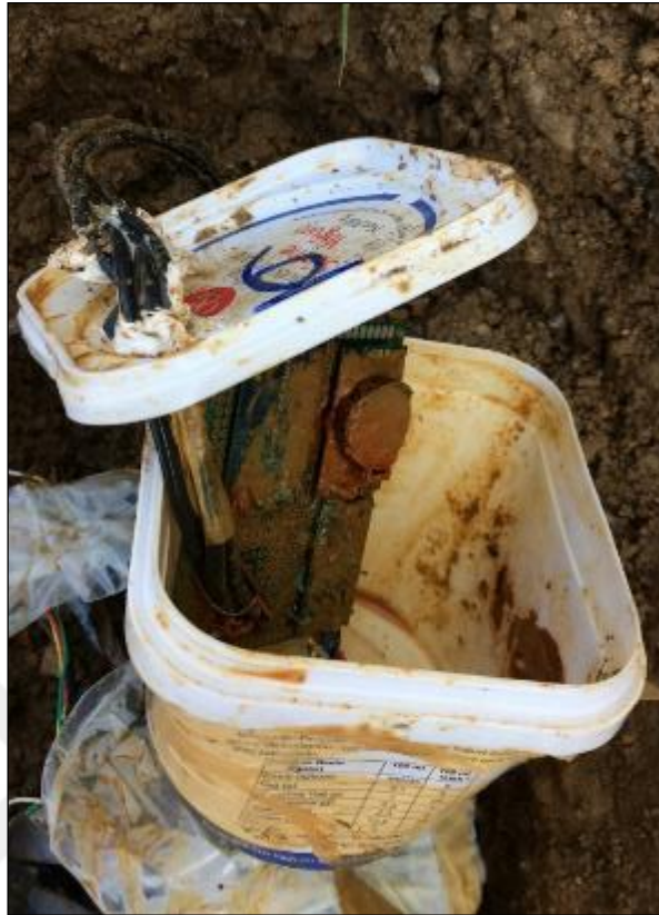
Figure 5.26. Location 3, Benzinlik, water damage.
