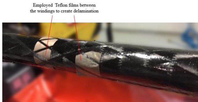
Figure 5.8 Insertion of teflon films during the filament winding process to create delamination
